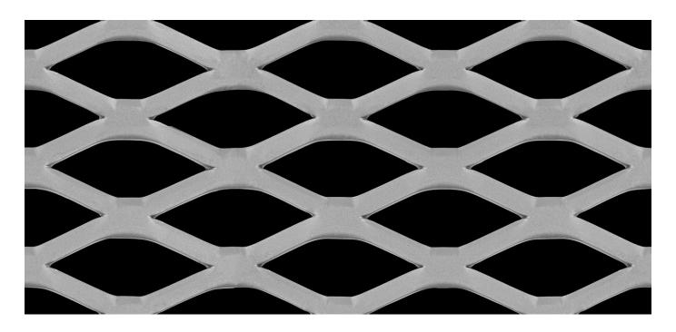
LW Aperture:43.00mmStrand Width:6.00mmSW Aperture:17.00mmThickness:4.00mmWeight:13.16 kg / m2Open Area:59%
